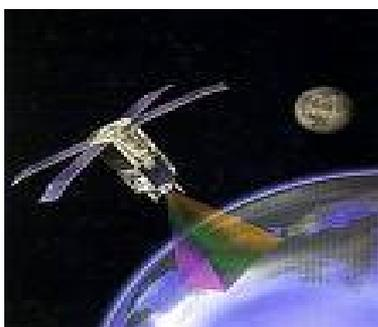
All the transmission media we have discussed so far have used a physical line to carry the transmitted information. However, data can also be transmitted using electromagnetic (radio) waves through free spaces as in satellite systems. A collimated microwave beam, onto which the data is modulated, is transmitted to the satellite from the ground. This beam is received and retransmitted to the predetermined destination(s) using an onboard circuit known as a
