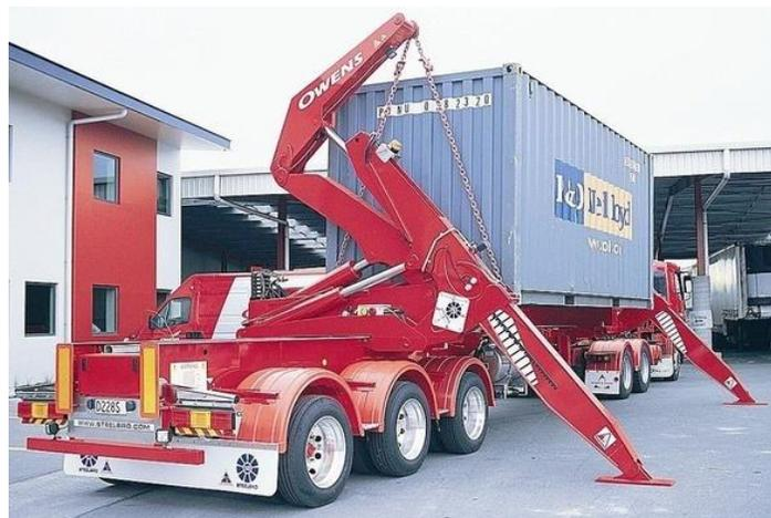
Figura 1.4 Grúa Sidelifter. Fuente. (Cranes and Machines, 2022)
