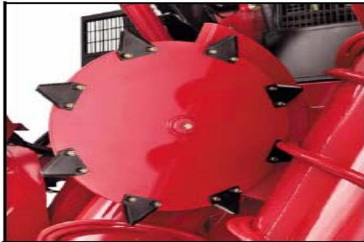
**Fig. 1.5 Discos de Corte Lateral (OPC)**
