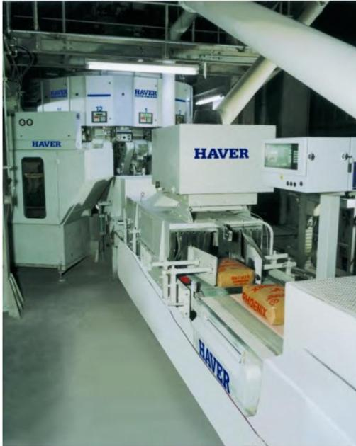
A Haver packing system with a Haver ROTO-PACKER, automatic bag applicator RADIMAT and check weigher
