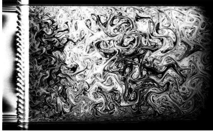
Figure A.4: Further increase in Reynolds number will make the flow turbulent, and there is a “stretching” of vortices
