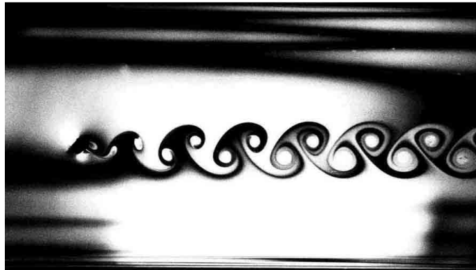
Figure A.2: A von Kármán street is created below the bolts at low Reynolds number
