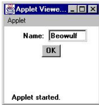
Figure 9.8: A narrower applet using Flow layout manager
