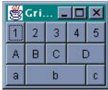
Figure 9.36: GridBagLayout example using RELATIVE/REMAINDER shorthands
