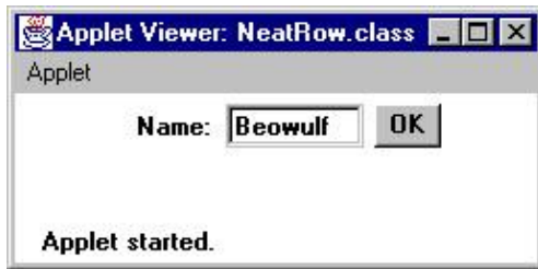
Figure 9.7: Simple applet using Flow layout manager
