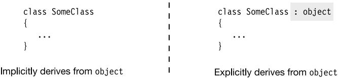
Figure 7-2. Direct inheritance from object
