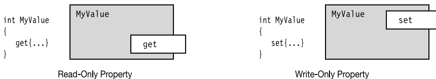
Figure 6-10. A property can have one or the other of its accessors undefined.
