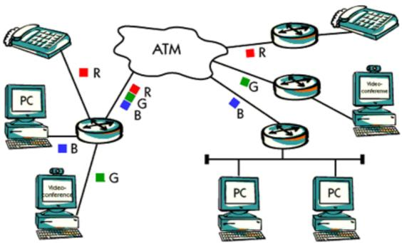
ATM, which stands for Asynchronous Transfer Mode is a "de facto standard" developed by the ATM Forum and is a switching method of communication, which can be used in both LANs and WANs.
