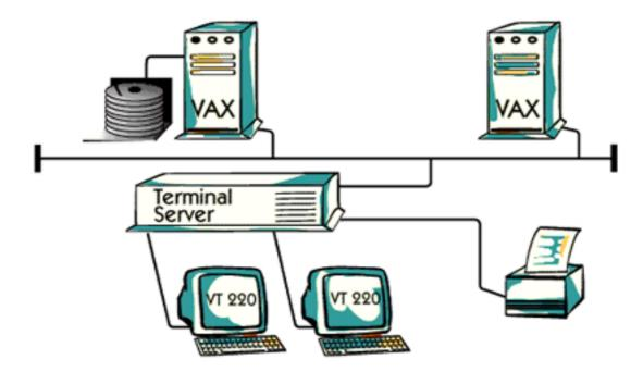
Ethernet, as defined in IEEE 802.3 standard, can use both star and bus topology with bandwidths between 10 and 100 Mbps. Ethernet is today the most common technique used in Local Area Networks.
