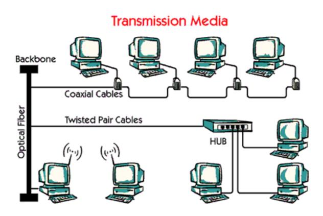
IEEE standards for LANs describe different types of transmission media. It could be cable, fiber or wireless.
