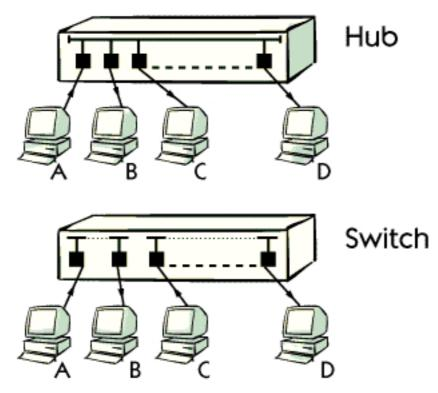
A hub is a commonly used device for connecting hosts to each other, using bus or ring topology. Each host is attached to a hub via a port. When a hub receives a signal on one port it transmits that signal to all other ports. Many hubs also regenerate and amplify weak signals before re-transmitting them.
