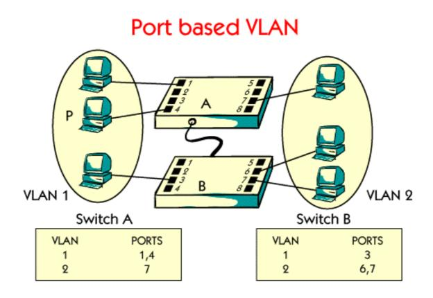
There are a number of different sollutions to create VLAN. Port based solution means that a host belongs to a particular VLAN based on which physical port in the switch the host is connected to. For example, the host P in the picture is connected to port 4 of switch A, which means that host P belongs to VLAN 1, as can be seen in the left table.
