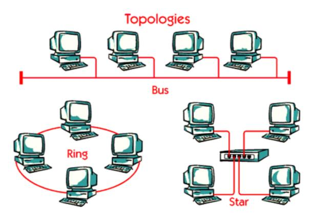
The topology of a network concerns the physical configuration of the devices and the cables that connect them.
