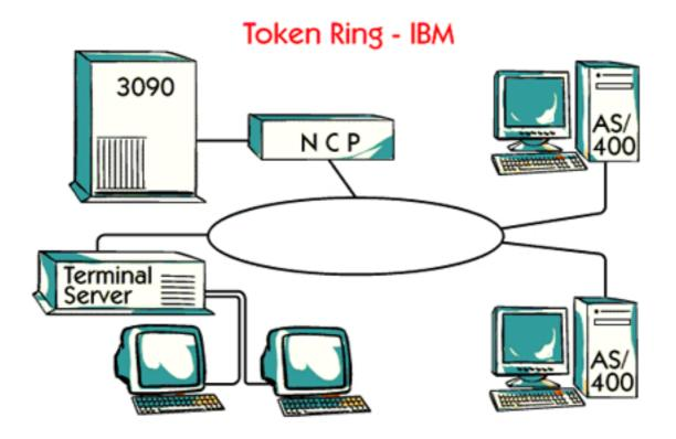
In this picture we see an IBM implementation of Token Ring. An IBM mainframe 3090 cannot directly communicate with the Token Ring. To do that it needs an NCP which is a dedicated computer that only handles the communication between the mainframe and the Token Ring network.
