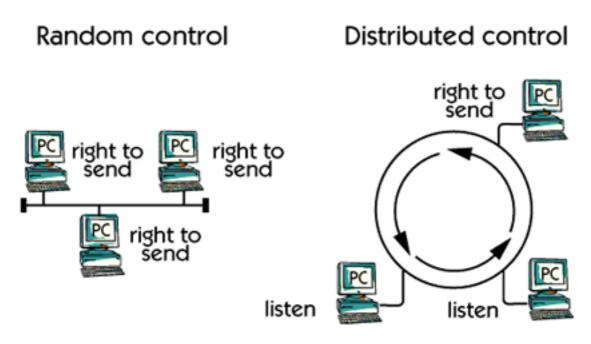
A characteristic common to all Local Area Networks is that multiple hosts have to share access to a single physical transmission medium. Several methods can be employed to control the sharing of access to the transmission medium.
