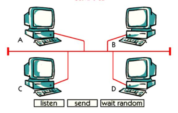
**CSMA/CD** stands for "Carrier Sense Multiple Access with Collision Detect". **CSMA/CD** is a random control access method.
