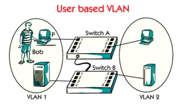
In the future there will be other VLAN solutions. One promissing solution, that many poeple wait for, is user based VLAN. When a user logs on a particular host, the user identity is anylized by the switch and then the host becomes a part of a particular VLAN. For example, the user Bob logs on the host P in the picture with his own user ID and password. The switch A decides that Bob belongs to VLAN 1.
