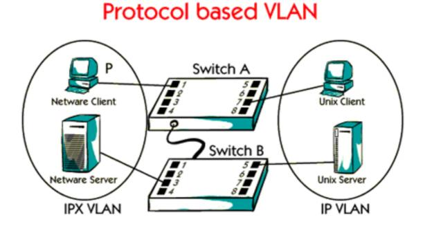
Protocol based VLAN means that a host belongs to a particular VLAN based on which protocol it uses for communication. For example, the host P in the picture is a Netware client which normally uses IPX protocol, which means that it belongs to IPX VLAN.
