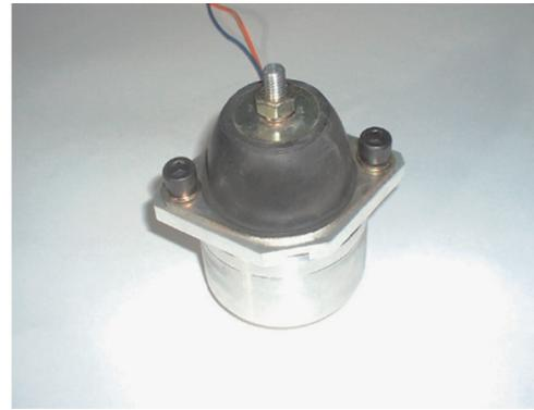
**Figure 46.** Schematic configuration and photos of the MR mixed-mode mount.
