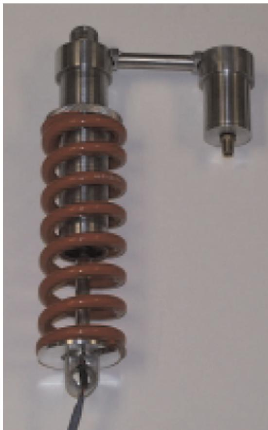
**Figure 39.** UNR-MRD-B2 rear damper around by coil spring.
