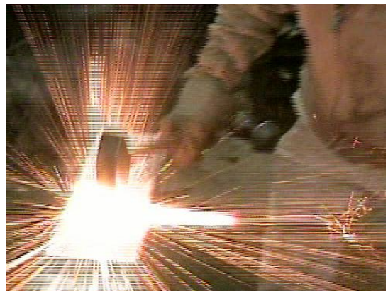
Fig. 1d) Forge-welding two 64 layer pieces together to create a 128 layer bar
