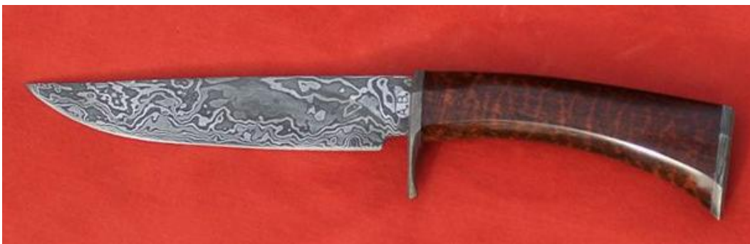
Fig. 2) 64 layer pattern-welded blade made of W-2, 203 E, and iron-nickel meteorite. Wrought iron guard and end cap, with snakewood handle. Forged by Tom Nizolek.
