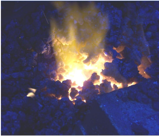
Fig. 1a) Heating a small piece of steel in a coal fire
