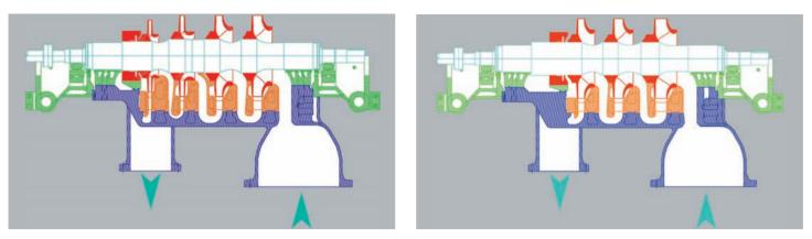
**4** Original 4-stage compressor and new aero bundle with 3 stages in the same casing (right).
