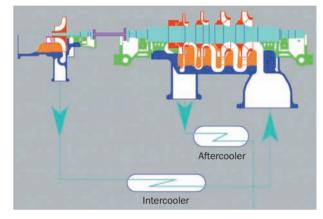
**5** Booster compressor with inlet guide vanes and intercooler added to the original compressor train.
