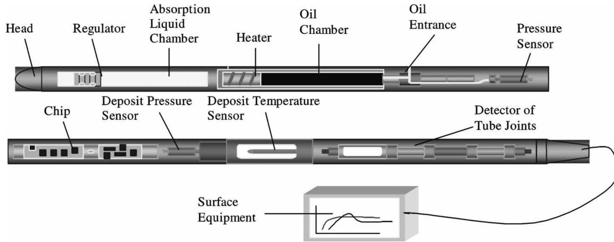
Figure 2. General scheme of sampling system.
