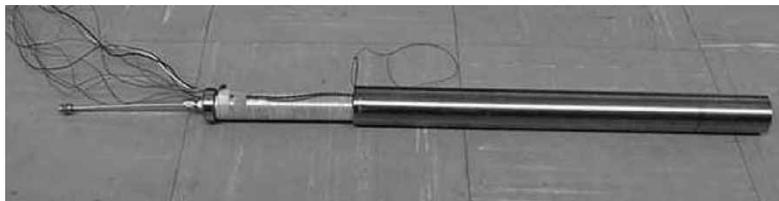
Figure 5. The heater and the container.
