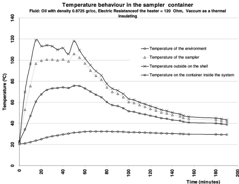
Figure 8. Temperature behaviour in the sampler container with optimum parameters.
