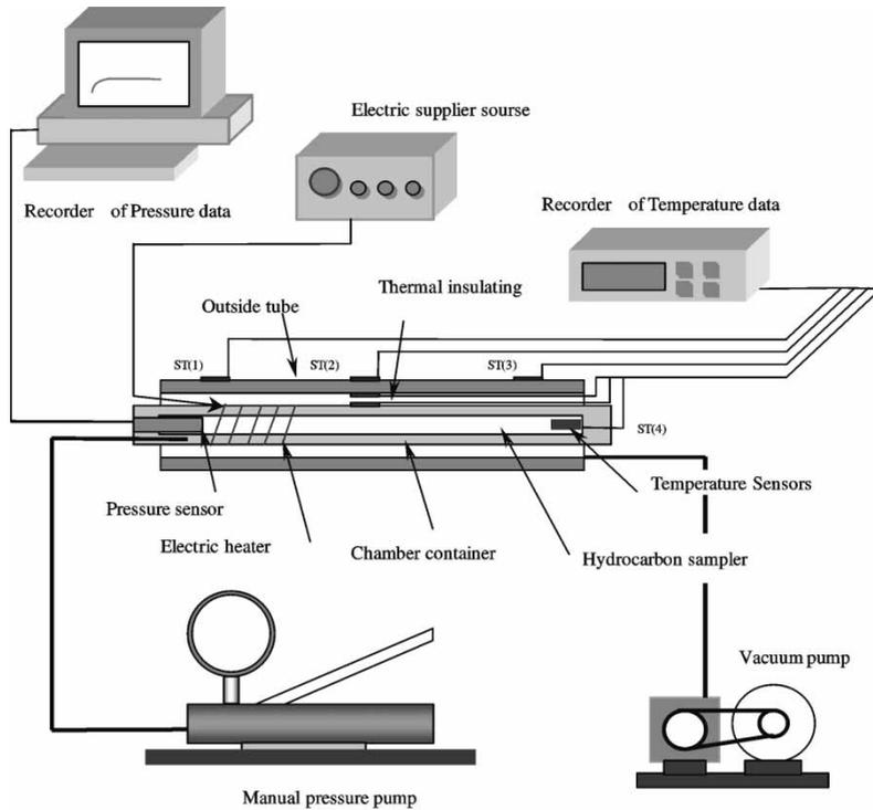
Figure 4. Whole system used to carry out the experiments.
