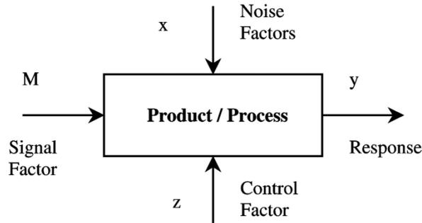
Figure 1. Block diagram of a product/process.
