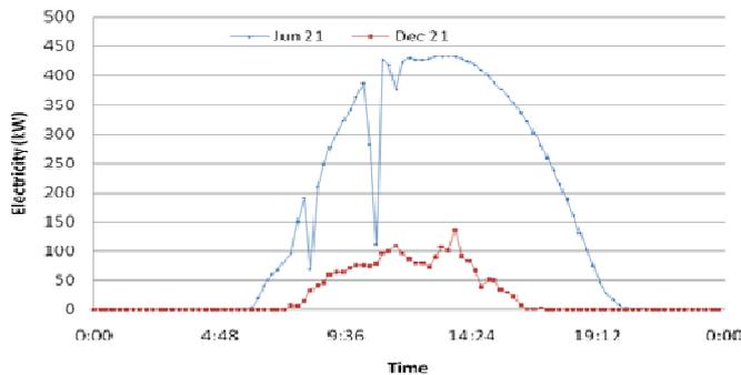
Figure 4. Electricity generation for a typical day in December and July
