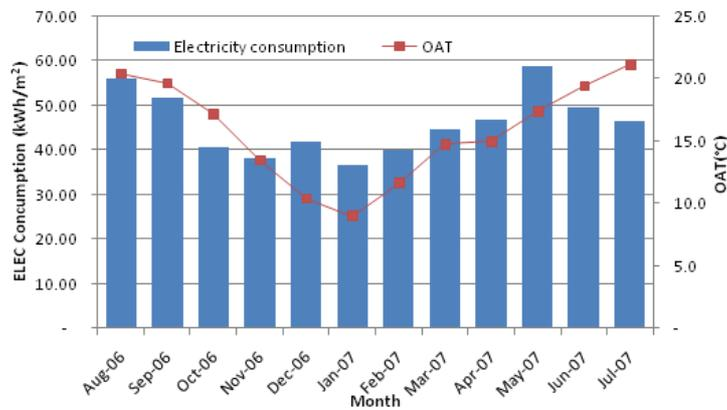
Figure 1. Monthly electricity consumption in FY06-07
