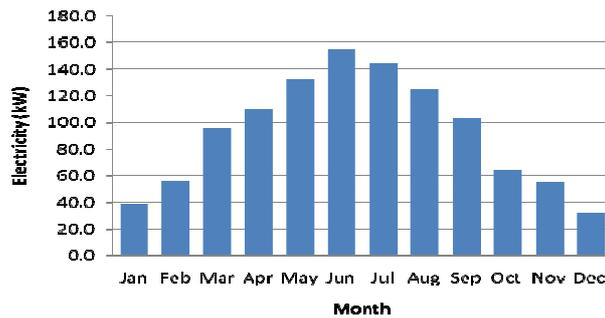
Figure 3. Average monthly electricity demand generated by the solar roof
