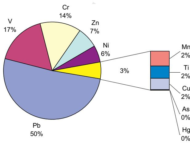
Fig. 4. Heavy metals composition of bottom ash from Cienfuegos oil refinery.
