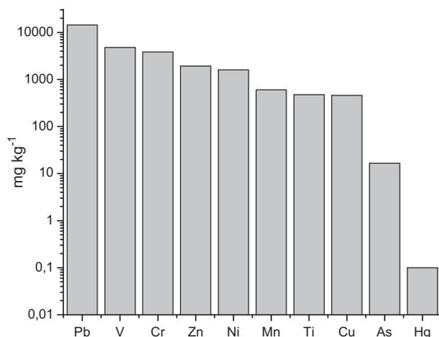
Fig. 3. Levels of heavy metals in bottom ash from oil refinery, Cienfuegos.
