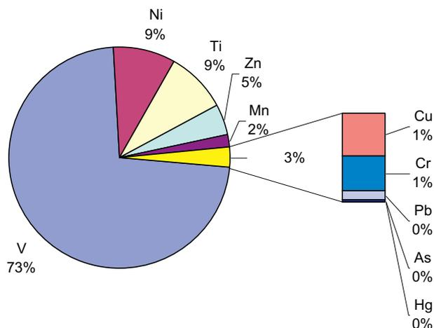
Fig. 2. Heavy metals composition of bottom ash from Cienfuegos power plant.
