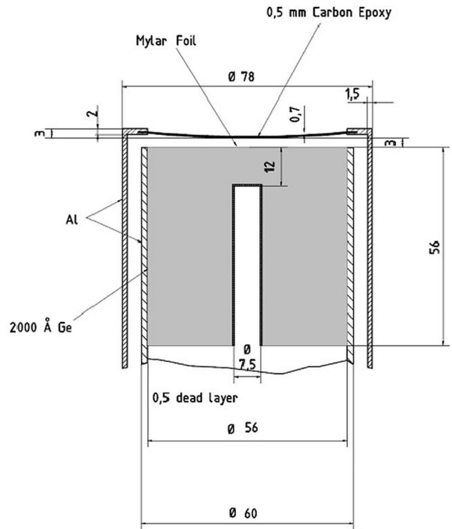
Fig. 1. Cross-section of the detector with the dimensions and materials provided by the manufacturers.
