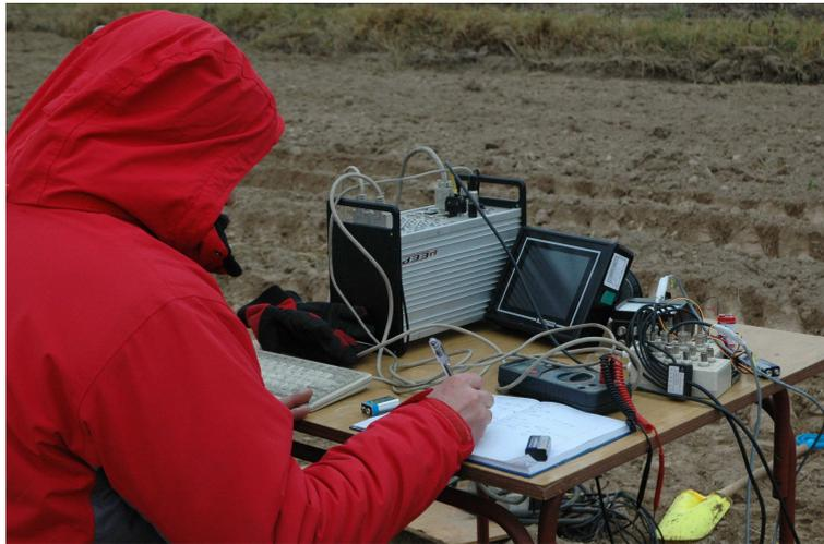
Fig. 4 Data acquisition computer
