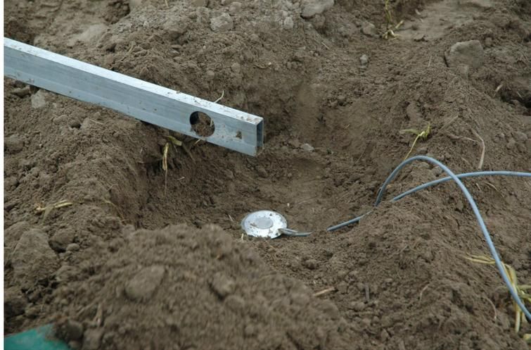
Fig. 3 Installation of the low profile sensor in soil
